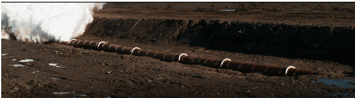
Figure 3-3 Large-scale testing of running ductile fracture in dense phase CO 2 . Picture from the CO 2 SafeArrest JIP.
