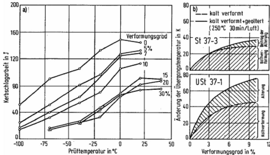
Figure 2: Charpy impact energy versus prestrain taken from [7]
