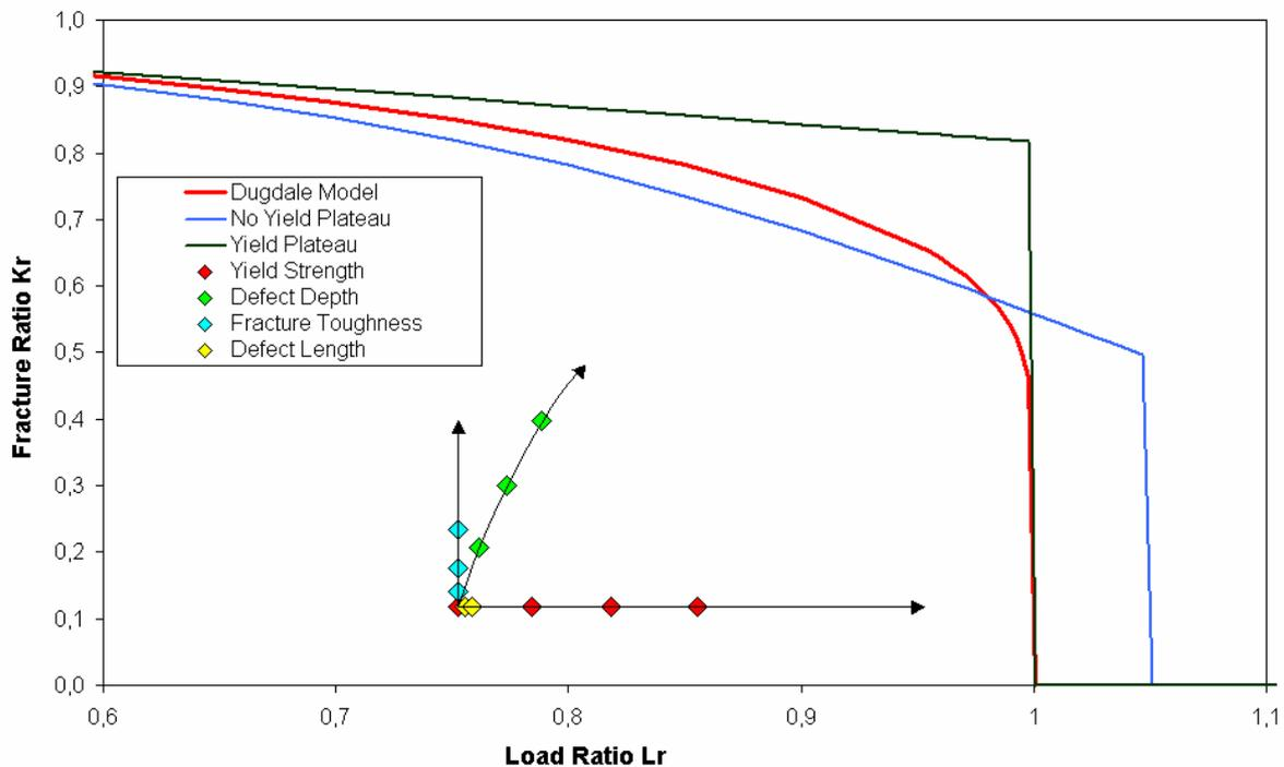
**Figure 1:** The FAD shows how the assessment point of a defect changes if the various input parameters are changed by one standard deviation per depicted point. The standard deviation is estimated from a probable distribution of these values. It is obvious that the yield strength and the defect depth can have quite an influence.
