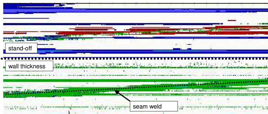
**Figure 3: C-Scan of the inspection data of an ultrasonic wall thickness measurement.**
