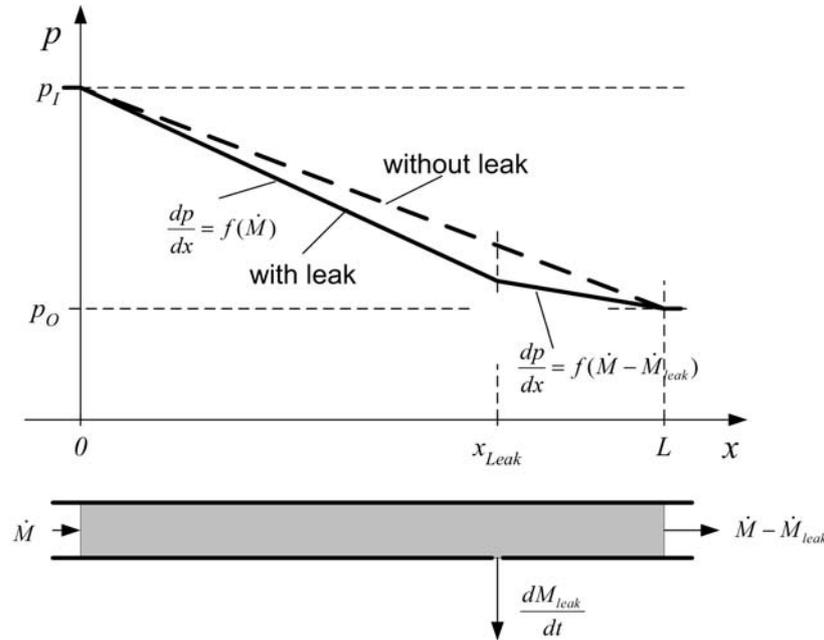
Measuring the straight line gradients (assuming that the friction factor  $f$  is known and estimates of the leak rate  $\dot{M}_{leak}$  are available) and calculation of the point of intersection therefore allow for leak location estimation [24].
