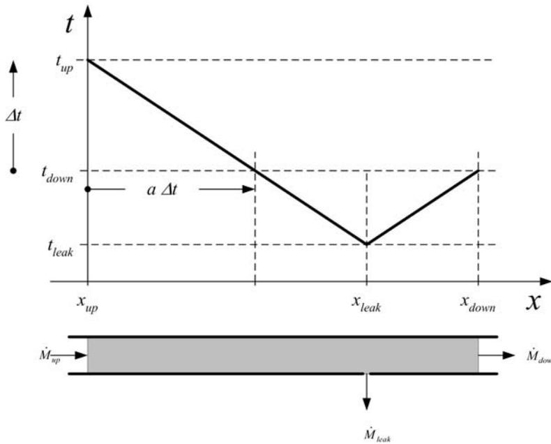
Time difference determination  $\Delta t \equiv t_{up} - t_{down}$  (assuming pressure transducer locations are known) gives the leak location estimate.
