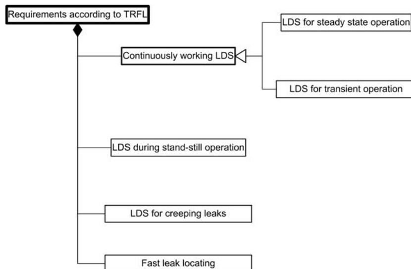
The TRFL is divided into the two parts “Operation” and “Constitution” of pipeline systems. Only a small part is concerned with leak detection and localization, focusing to the specification of measures necessary in order to detect and locate leaks. Five different LDS and LDS functions are required<sup>1</sup>, see Figure 1:
