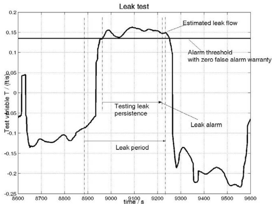
A test variable  $T$  is tested against an alarm threshold  $A$ .  $T$  exceeds  $A$  shortly after leak occurrence; now, testing leak persistence within the scope of outlier removal procedure starts. Leak alarm is raised after leak persistence has been confirmed.
