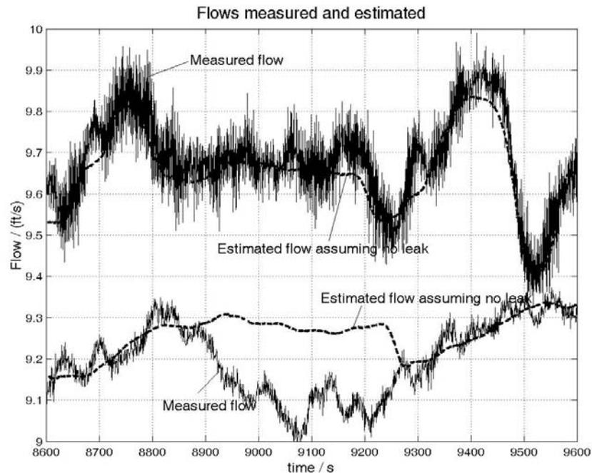
Due to the deviation principle, significant deviations between measured and estimated flow indicate a leak in the pipeline, which occurs for the application at time  $t=8900$ s. Results of the leak signature analysis are shown by the next figure.
