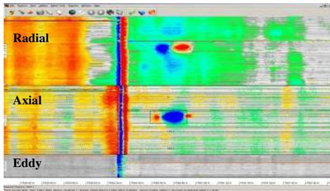
Figure 2: MFL data of a metal gain, most likely a metal object
