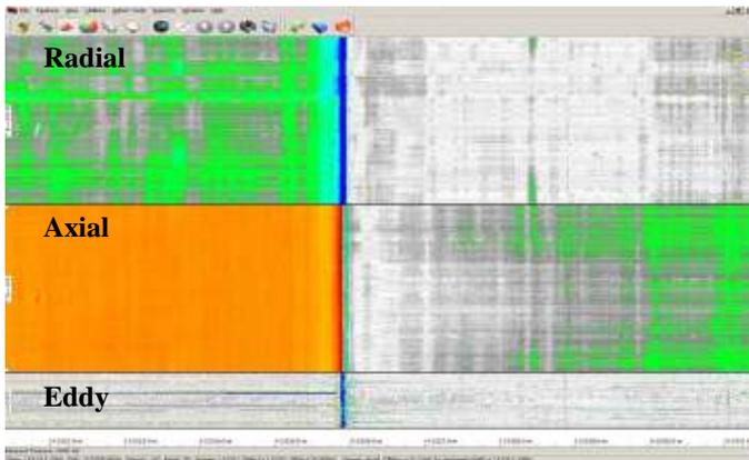
Figure 13: MFL data of a wall thickness change
