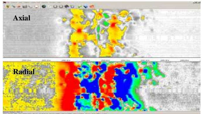
Figure 4: MFL data of a highly corroded complex area
