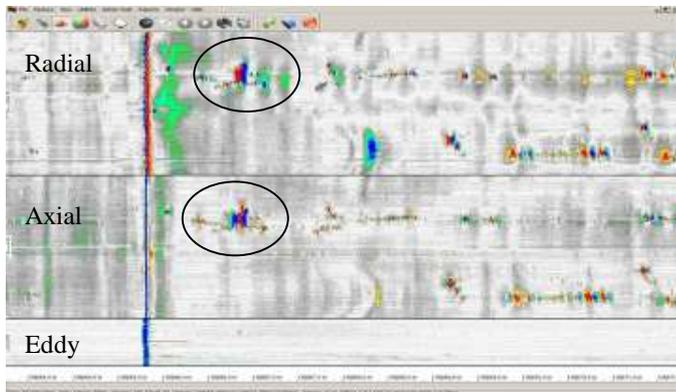
Figure 6: MFL data of an area containing complex corrosion
