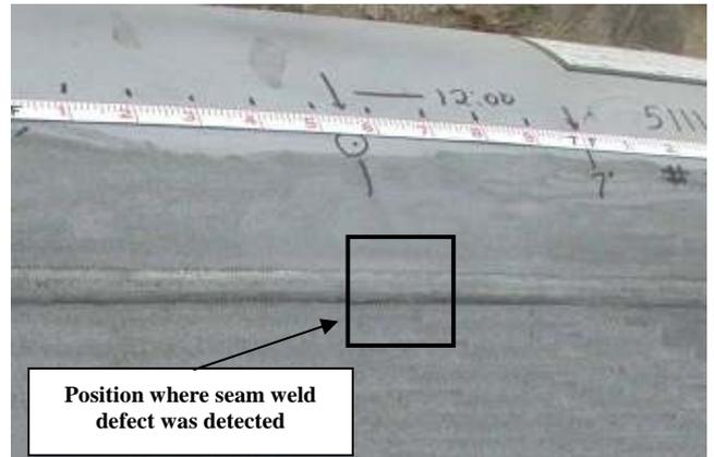
Figure 29: Photo of an apparent corrosion on a seam weld
