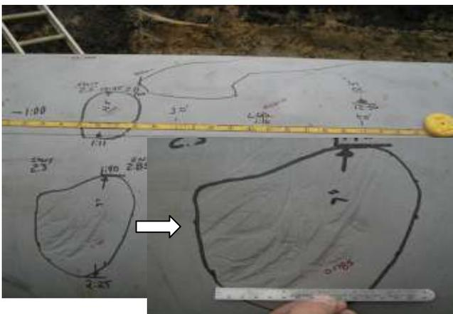
Figure 36: Photo of a Gouging without Denting
