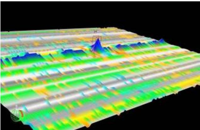
Figure 28: Radial (above) and Axial (below) MFL data of apparent corrosion on a seam weld
