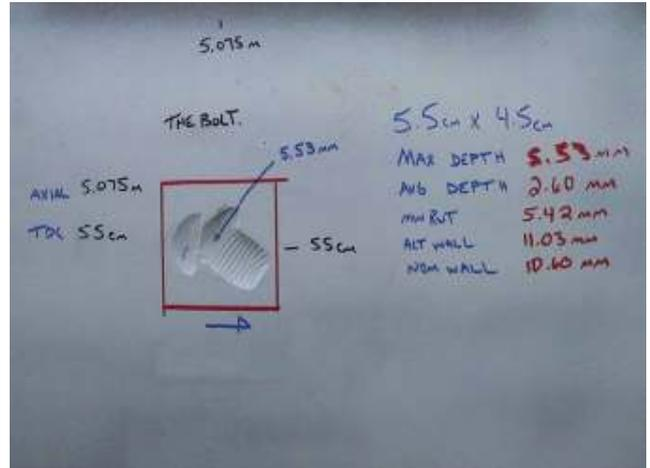
Figure 26: Photo of a metal loss from a steel bolt imprint
