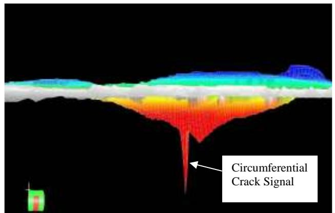
Figure 38: Radial oriented MFL data of a crack in a dent
