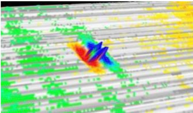
Figure 25: Radial (above) and circumferential (below) MFL data of construction damage
