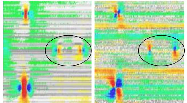
Figure 8: Axial and Circumferential sensor data of three defects.
