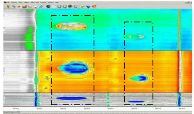
Figure 11: MFL data of a Tee (left) and port (right)
