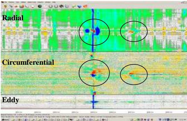
Figure 32: Radial, Circumferential and Eddy MFL data of a dent
