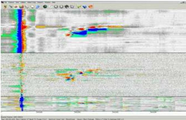
Figure 35: MFL Data of a gouging without denting
