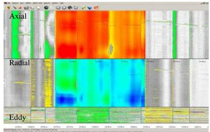
Figure 16: MFL data of a casing
