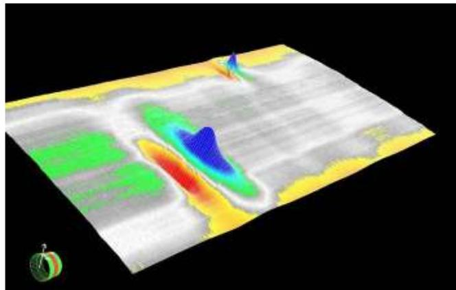
Figure 1: MFL data of the radial oriented sensor of two defects with different signal amplitudes
