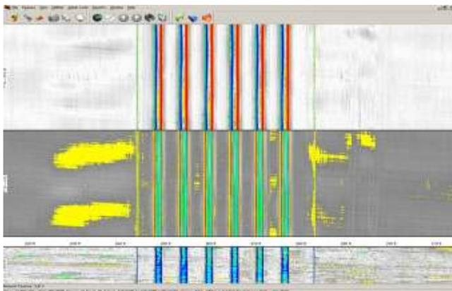
Figure 18: MFL data of a mitre bend (above), and graphical display of the inertial data (below)
