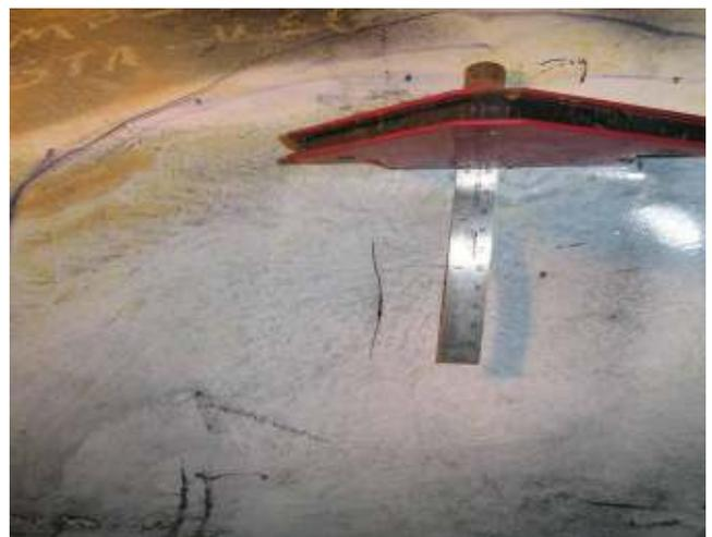
Figure 39: Photo of a large crack inside a dent identified by an MFL Inspection tool
