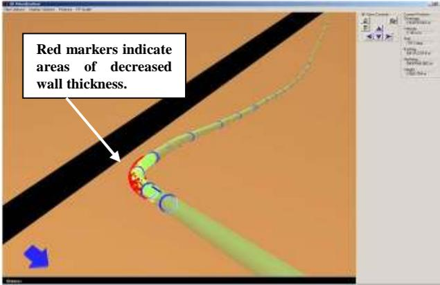
Figure 20: Graphical display of the inertial data
