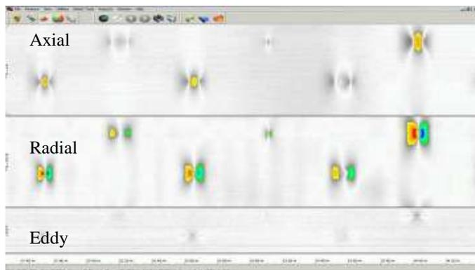
Figure 3: MFL data of 6 separate metal loss features
