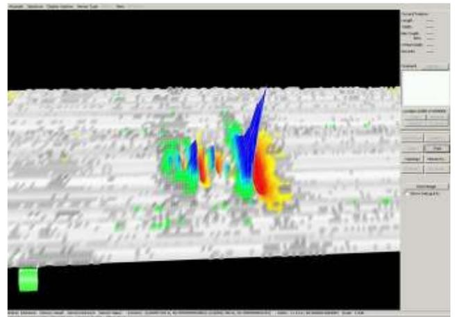
Figure 23: MFL data of a defect
