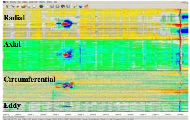
Figure 37: MFL data of a dent with a crack at its center
