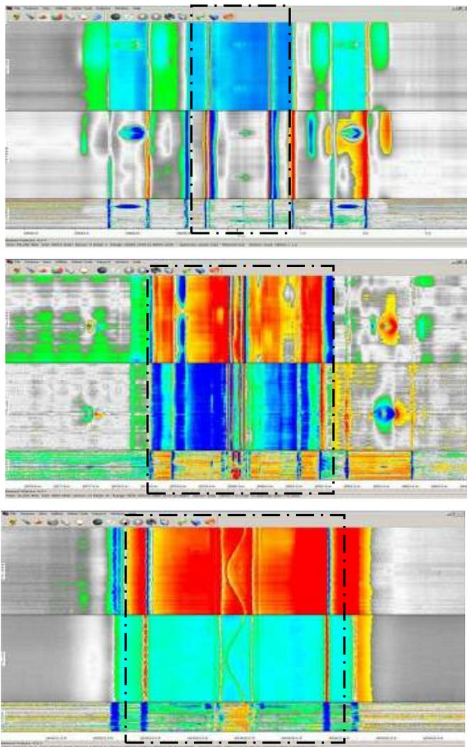
Figure 10: MFL data of three different valve types
