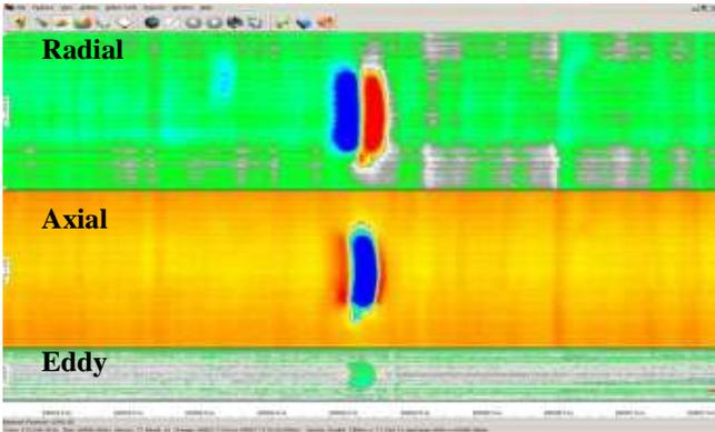
Figure 17: MFL data of an anchor (above) and a support (below)
