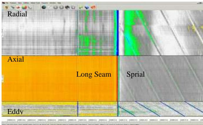
Figure 14: MFL data of Long Seam vs. Spiral Weld
