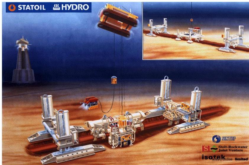
Figure 2 PRS welding habitat during installation for welding at the Langeled pipeline.
