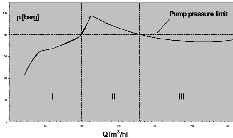
Table 3 shows the maximum operating parameters for each of the three pumps installed. While during phase I of figure 3 it is sufficient to run only one pump, two pumps are operating in parallel during phase III. For phase II two pumps would work in series, while the third pump always is kept stand-by. However as can be seen in the simplified P&I diagram (fig. 4), all available pumps can be placed in the respective process flow as may be needed.
