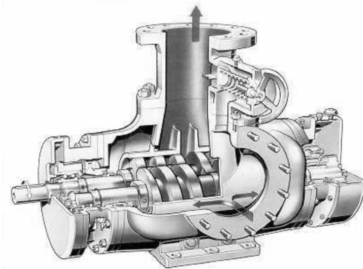
As the pump only transfers a volume from suction to discharge, no pressure is created internally. Just a response to the downstream backpressure is given. An integrated spring loaded relief valve prevents the pump from being over-pressurized. It allows for an internal circulation in case of backpressure being too high.
