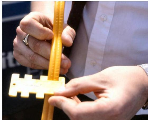
The size and shape of the bead can indicate error with procedural factors and raise alarm about the quality of the joint.
