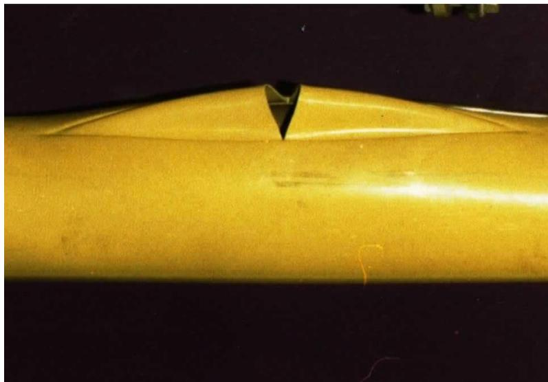
Failure Mode II is associated with Creep, Creep Rupture and SCG. Creep is time-dependant, non-reversible deformation, when exposed to a constant tensile stress. Creep rupture is the terminal event of creep and is a measure of the time that a material under a constant, applied tensile load takes to fail.
