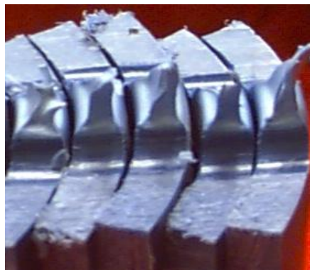
Figure 19 Mixed Mode Failure (Top) and Brittle Failure (Bottom)
