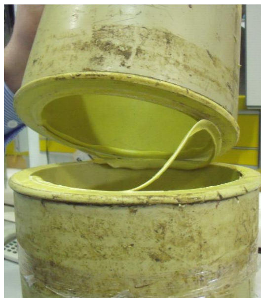
Figure 9 Catastrophic Failure of Butt Fusion Joint
