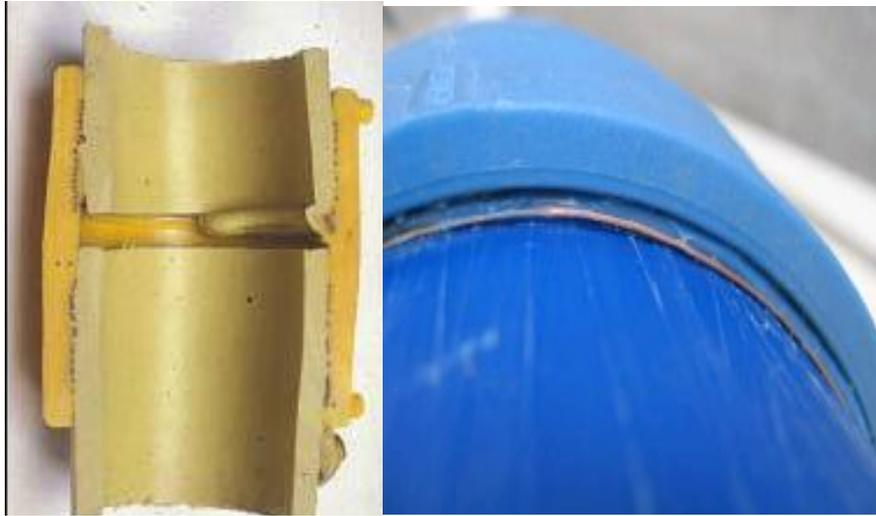
Contamination is also a major issue that can lead to premature failure of electrofusion joints. It is generally associated with the surface of PE pipe because of the way it is transported, stored, handled etc. However, two surfaces are required to make a joint and sometimes the condition of the fitting surface is forgotten.
