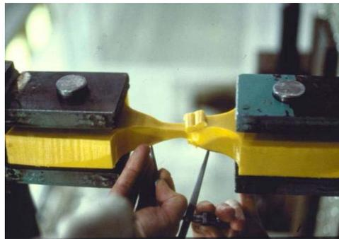
**Figure 18** Ductile Failure
