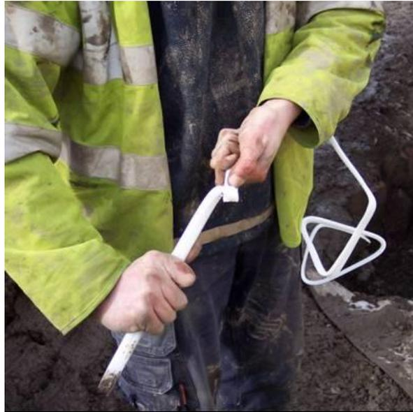
The bend back test can also be used to detect poor fusion, which will result in bead separation. Examination of the underside of the bead over its complete length also allows detection of general contamination.
