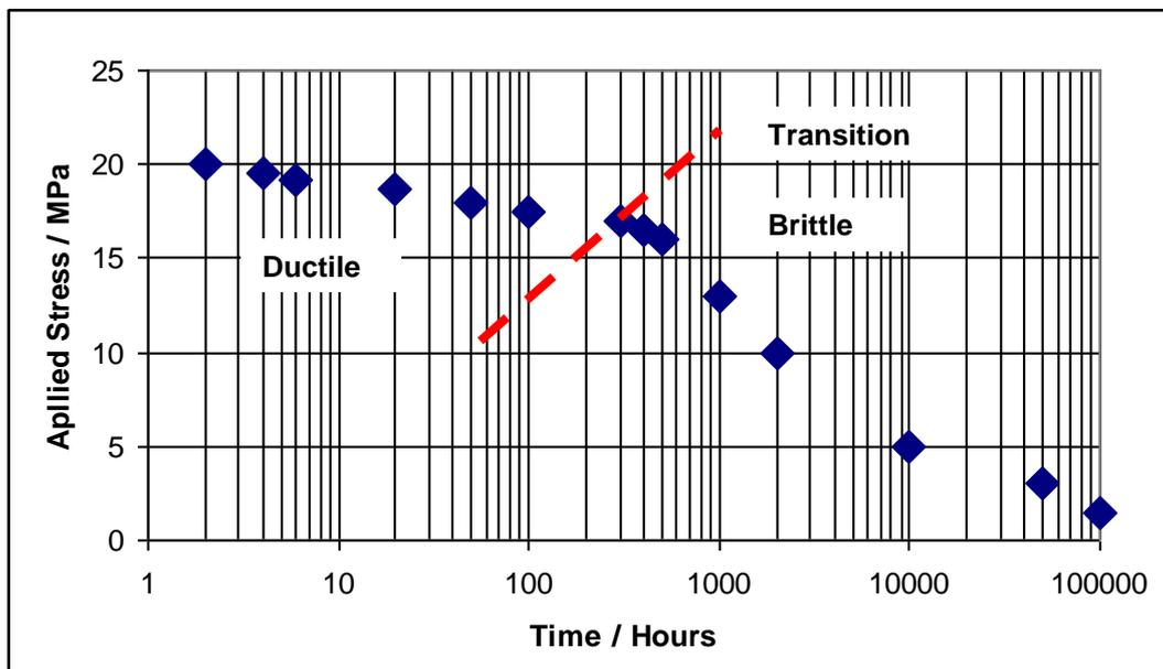
The events that lead to Creep Rupture are shown in Figure 5.0. After crack initiation voids develop ahead of the crack. These voids gradually merge into larger voids that are spanned by highly orientated load bearing fibrils. This process known as Crazeing continues until a point is reached when the most highly stretched fibrils will rupture resulting in fracture.
