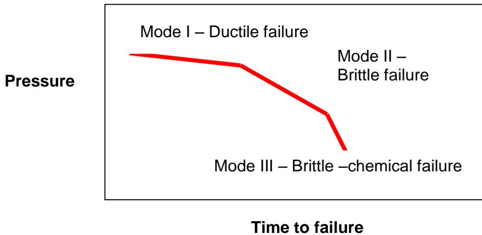
Ductile failure mode I, results in yielding and reflects a material's propensity to undergo large-scale, irreversible 'plastic' deformation when under stress. The mechanism results in localized expansion of the wall section and final rupture of the deformed zone as shown in Figure 3.
