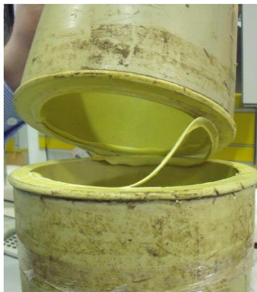
**Figure 10** SCG Preceding Catastrophic Fracture of the Complete Joint
