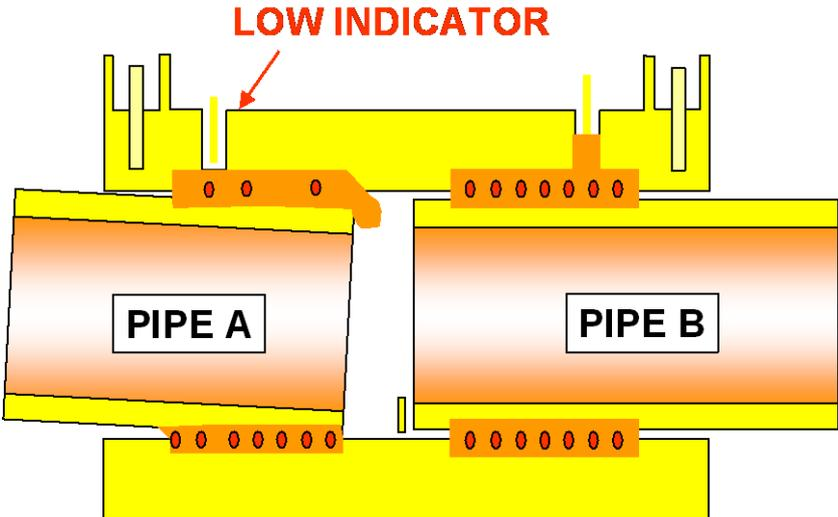
**Figure 22** Consequences of Incorrect assembly
